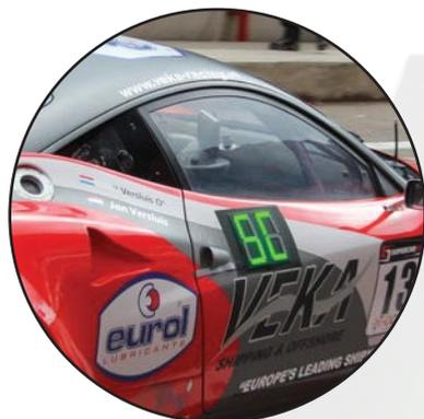
Spectators can now view the car positions live with the SPAA05 Race Position Display! See who is in front, even in long endurance races with 255 cars. The RPD system fits all cars with 2 large 30x21 cm displays with bright and fully coloured LED lights that show the race position of the car.
